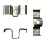
Grating Fasteners Model "**SSI-60**" is a 316 Stainless steel grating fastener used to fasten pultruded fiberglass grating to structural shapes. This particular fastener is installed with a tek screw.
