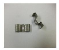
Grating Fasteners Model "**SSGF-1.5**" is a 316 stainless steel grating fastener used to fasten 1-1/2" square mesh fiberglass grating to structural shapes. This particular fastener can be installed with a tek screw.
