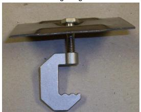
G-Clip TM model **FFSCGC-** is a 316-stainless steel grating fastener used to fasten fiberglass T-bars to structural members. Like many of our other G-Clips, they are for use where the structural flange is in a horizontal plane. Other stainless steel tops are available for use with the SCGC gripjaw, to be used on popular pultruded and molded fiberglass gratings with a minimum of 3/8" opening.
