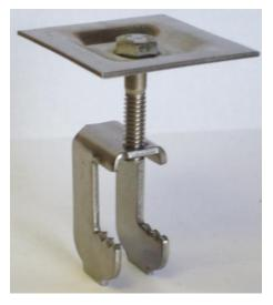
G-Clip ™ model **YSSGG-** is a 316-stainless steel grating fastener used to fasten 1.5" square mesh fiberglass grating to metal structural shapes, where the structural flange is in a horizontal plane. The specially shaped top is designed to fit 1.5" square mesh fiberglass gratings.
