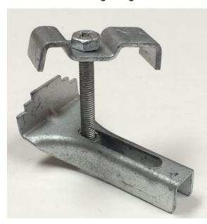
Grating Clip model **BCGC-516** is a galvanized carbon steel grating fastener used to fasten steel bar grating to structural shapes where the structural flange is in a horizontal plane. For appropriate use, the maximum measure from the top of the grating to the bottom of the flange is 2.5 inches. It can be used on 22-spaced grating and 30-spaced grating. It will work on 19-spaced grating, but note that the grating bars will spread during tightening.
