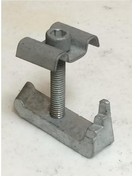
Grating Clip model **GSLF-38** is a galvanized steel grating fastener used to fasten standard steel bar grating to structural shapes where the structural flange is in a horizontal plane. For appropriate use, the maximum measure from the top of the grating to the bottom of the beam flange should be 2" or less. It is designed to be used on 19-spaced grating with bearing bars from 1/8" to 1/4" wide.
