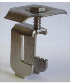
G-Clip <sup>™</sup> model **WSSGG-** is a 316-stainless steel grating fastener used to fasten bar grating to metal or other structural shapes, where the structural flange is in a horizontal plane. Other stainless steel tops are available for use with the SSGG gripjaw, to be used on popular pultruded and molded fiberglass gratings.
