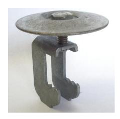
G-Clip ™ model **RGN-** is a galvanized carbon steel grating fastener used to fasten odd-spaced gratings to structural members, where the flange is in a horizontal plane.
