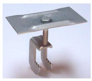
G-Clip TM model **FFGN-** is a galvanized carbon steel grating fastener used to fasten grating with wide spaced bars, typically 38-space. Like many of our other G-Clips, they are for use where the structural flange is in a horizontal plane.
