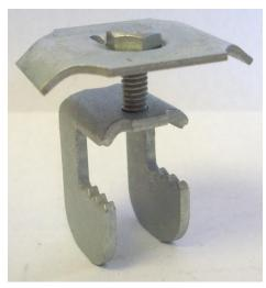
G-Clip ™ model **GG-0** is a galvanized carbon steel grating fastener used to fasten 1" high 19-space bar grating to minimal-thickness structural member edges. The GG-0 will clamp 1" grating to beam edges as thin as 0.05". In some cases, the GG-0 will also work for 0.75" tall gratings
