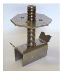
G-Clip ™ model **SSGM-1/2**" is a stainless steel fastener used to fasten lightweight devices to 19-space bar grating. The SSGM-1/2" is designed to be used instead of J-bolts. It will withstand 1000 pounds of direct upward pull force. Due to its 316SS material, it can be used in corrosive environments.
