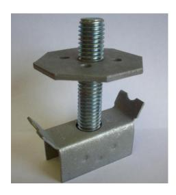
G-Clip ™ model **GM-1/2**" is a fastener used to fasten lightweight devices to 19-space bar grating. The GM-1/2" is designed to be used instead of J-bolts. It will withstand 1000 pounds of direct upward pull force.
