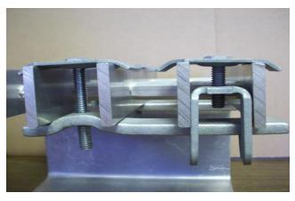
G-Clip <sup>™</sup> model **GP-** is a galvanized carbon steel fastener used to fasten parallel sheets of 19space bar grating together. The purpose of the GP- is to prevent deflection due to weight loads and eliminate trip hazards. It requires a companion model GG- to be installed correctly. They are sold either alone as GP's or in GP/GG sets. The installed GP/GG set is shown in the picture on the left.
