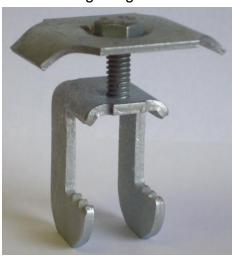
G-Clip TM model **GG-** is a galvanized carbon steel grating fastener used to fasten 19-space bar grating to structural shapes, where the structural flange is in a horizontal plane.
