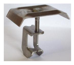
G-Clip ™ model **FSSGF-** is a 316-stainless steel grating fastener used to fasten pultruded bar grating to fiberglass or coated steel structural shapes, where the structural flange is in a horizontal plane. The specially shaped top is designed to fit pultruded grating shapes, while restricting the spreading of the bearing bars.
