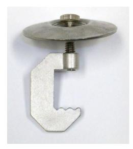
G-Clip TM model **RSCGC-** is a 316-stainless steel grating fastener used to fasten close mesh bar grating to metal or other structural shapes, where the structural flange is in a horizontal plane. The narrow grip-jaw on the clip allows it to be used on gratings with as little as 3/8" opening. Our nickname for this part is "Cast Close-Grip."
