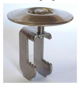
G-Clip ™ model **RSSGG-** is a 316-stainless steel grating fastener used to fasten odd-shaped bar grating to metal or other structural shapes, where the structural flange is in a horizontal plane. Other stainless steel tops are available for use with the SSGG gripjaw, to be used on popular pultruded and molded fiberglass gratings, or in highly corrosive environments.
