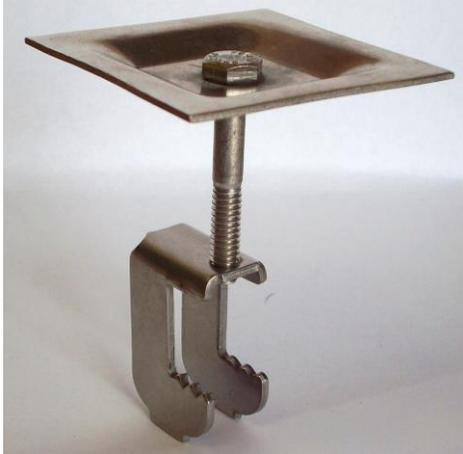
G-Clip™ model **ZSSGG**- is a 316-stainless steel grating fastener used to fasten 2" square mesh fiberglass grating to metal structural shapes, where the structural flange is in a horizontal plane. The specially shaped top is designed to fit 2" square mesh fiberglass gratings.
